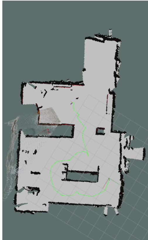
(b) Top-down view of the real-world path (green) the robot took to explore the scene in an episode of the ImageNav task with the point cloud from the robot's head camera and a 2D lidar map.
